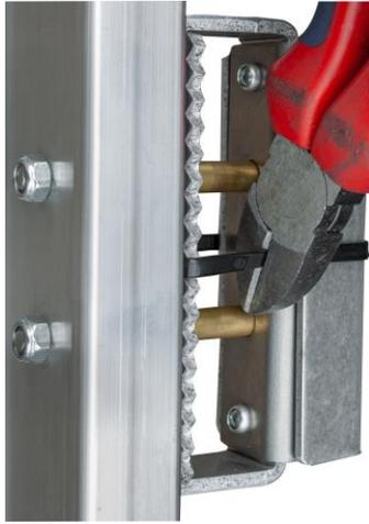
4. Now break and remove the cable tie.
