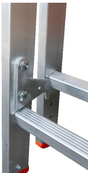
Segment hook not in place
