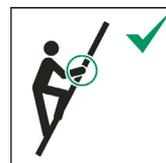
Keep a secure grip on the ladder when ascending and descending. Maintain a handhold whilst working from a ladder or take additional safety precautions if you cannot.
