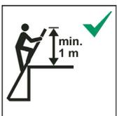
Ladders used for access to a higher level shall be extended at least 1 m above the landing point and secured, if necessary.
