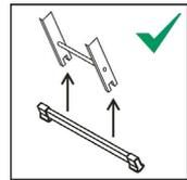
If a ladder is delivered with stabilizer bars and these bars should be fixed by the user before the first use this shall be described on the ladder and in the user instruction.
