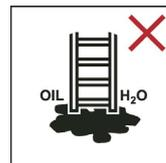
Do not erect ladder on contaminated ground.
