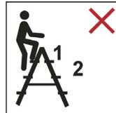
Do not stand on the top two steps/rungs of a standing ladder without a platform and a hand/knee rail.
